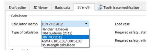
Also, shaft deformation and bearing force calculation, considering non-linear bearing stiffness, is included in KISSsoft. Beam theory, either as per Euler or as per Timoshenko is used. Linear or non-linear calculations are available. Several single shafts may be combined to form a – coaxial – shaft system.
