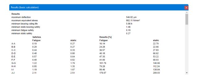
Resulting safety factors are reported for each cross section. Static and fatigue safety factors, as well as utilizations are reported.
